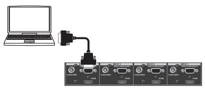
To assign RGB input to channel 4, go to [A-BUS/PGM] and press [4], then press the [RGB/COMPONENT] button. When the V-40HD detects the RGB input, the [INPUT STATUS] indicator of the channel 4 lights up.
