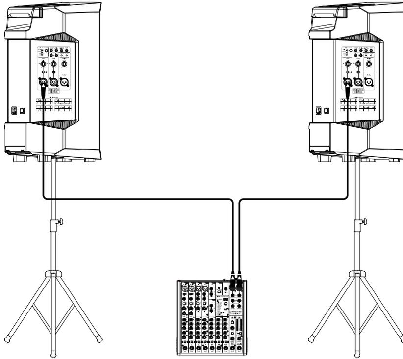
In this example, a ProFX10v3 mixer is connected directly to two Thump GO loudspeakers. It is the perfect setup for a small club. Simply connect the L/R outputs of the ProFX10v3 mixer to the channel 1 input of each Thump GO loudspeaker. The gain knob on both should be set to Line. Don't forget to set the Voicing Mode on both loudspeakers to 'Music'!
