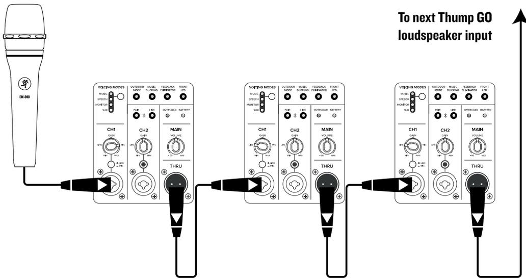
Thump GO loudspeakers may be daisy-chained via the male XLR connector labeled “THRU”. Simply plug the signal source (i.e., mixer output or microphone) into the input jack(s), and patch that loudspeaker’s thru jack to the next loudspeaker’s input jack, and so on, daisy-chaining multiple Thump GO loudspeakers. See above for visual representations of daisy-chaining.
