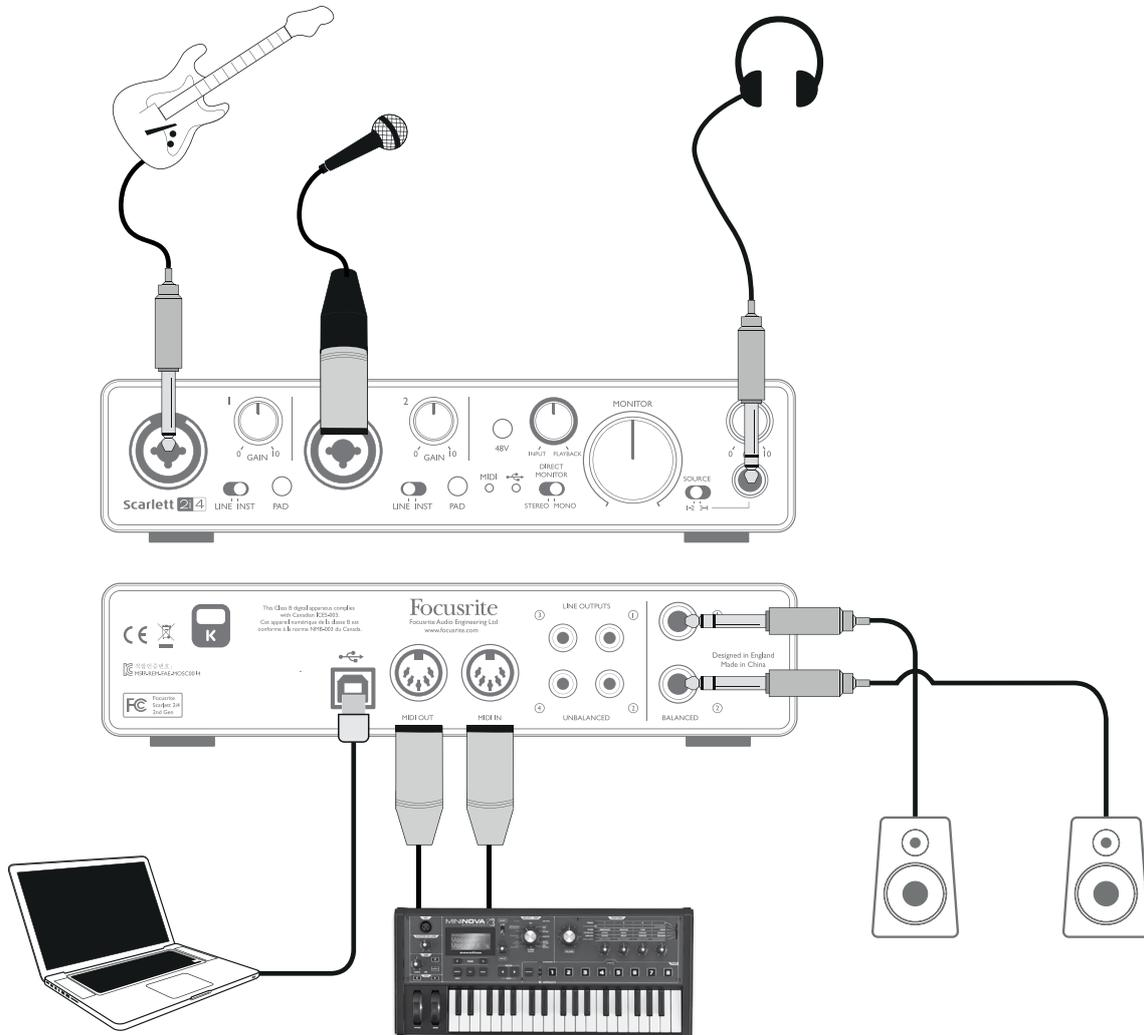
This setup illustrates the most typical configuration for recording with DAW software on your Mac or PC. In this case, you might record guitar through Input 1 and vocals through Input 2 into Ableton Live Lite, while monitoring the playback from the DAW via headphones or loudspeakers.
