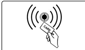
RFID card come with consumable HC8200 bags, swiping card to identify parameters and types of granules. The RFID card is disposable, one card can only use one time.
