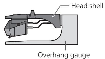
② Move the cartridge to line the stylus tip up with the end of the gauge.
