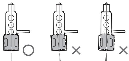
③ Tighten the screw for cartridge.
