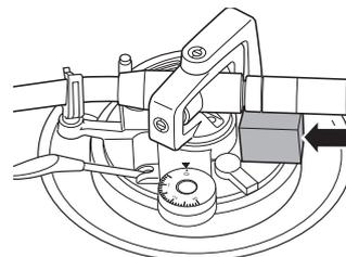
Before repackaging, remove the balance weight and insert the tone arm support under the tone arm.
