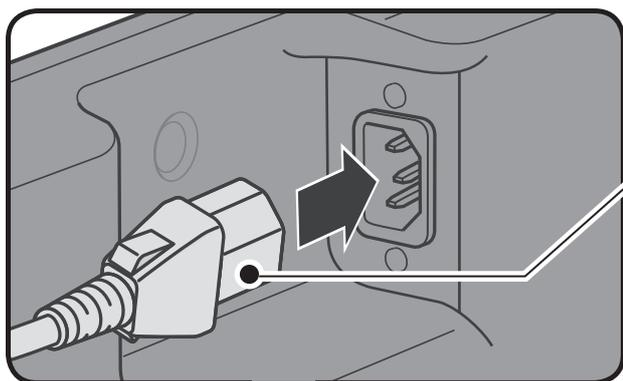
Insert the AC mains lead up to a point just before the round hole.
