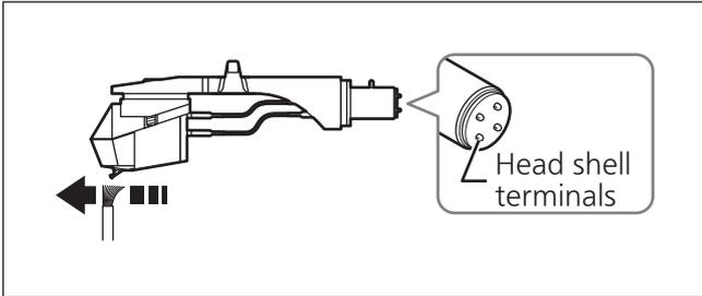
**Wipe the head shell terminals occasionally.** Wipe the head shell terminals with a soft cloth and fit the head shell to the tone arm.
