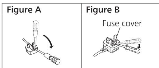
2. Replace the fuse and close or attach the fuse cover.
