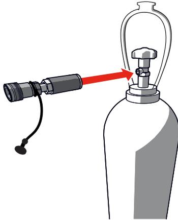
4. Connect the CO2 hose to the CO2 bottle-to-hose connector on the CO2 cylinder.
