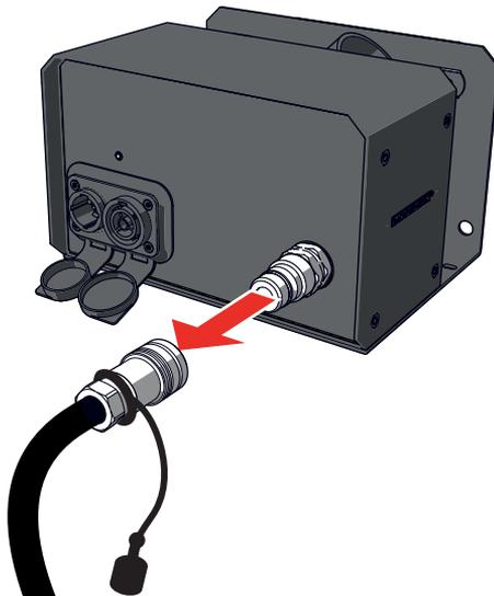
5. Disconnect the CO2 hose from the CO2 bottle-to-hose connector on the CO2 cylinder.
