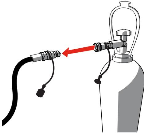
6. Remove the CO2 bottle-to-hose connector from the cylinder.
