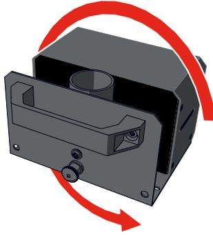
2. Screw a M10 twenty clamp for truss mounting (product code MFX3103) into both threaded holes.
