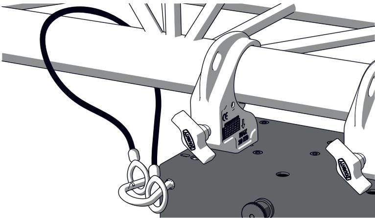
5. Inspect if the CO2 JET II is mounted firmly and secured correctly.
