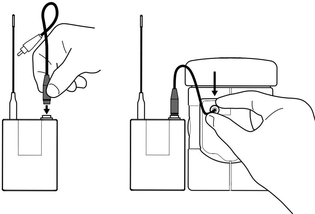
Afterwards, place the 3rd party transmitter inside the cavity of the Catchbox Pro Module, making sure no antennas or cables are protruding outwards.
