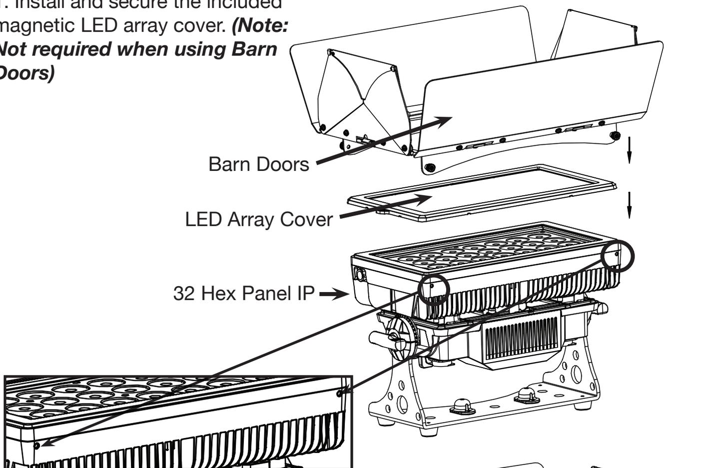
2. Place the Barn Door attachment over the front of the unit. Line up the 4 Barn Door thumb screws with the thumb screw holes located on each side of unit (2 on each side). Screw thumb screws in and tighten. **DO NOT** overtighten.
